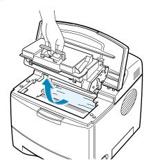
**CAUTION:** To prevent damage to the toner cartridge, do not expose it to light for more than a few minutes. Place a piece of paper over the top of the toner cartridge to shield it while it is out of the printer.
